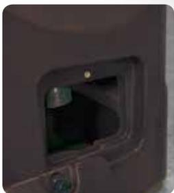
A double-walled cover gives access to the drain and protects it from the cold.
